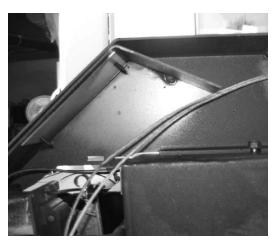
Remove Thermal switch from right hand fan mounting bracket and relocate to left hand fan mounting bracket. Fig #20&21
