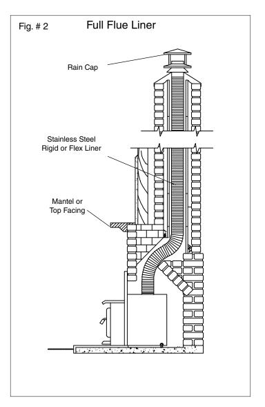
Pacific Energy highly recommends the use of a full liner as the safest installation and providing optimum performance. When connected to a full liner, the Insert is able to draft correctly and will prevent problems such as difficult start-ups and smoking out the door.
