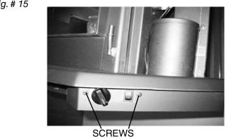
5) Remove the control assembly from the right hand side of the ashlip. Flip it over and reattach on the left hand side of the ashlip. Use the upper screw holes for best alignment.
