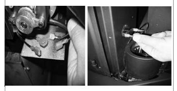
3) Loosen the two bolts that secure the ash lip to the firebox, carefully lift up the ash lip and remove from the firebox and unscrew the wire support tabs.
