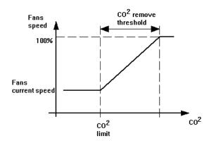
Function is activated using a *CO2 function* parameter. Before activating the function, the CO<sup>2</sup> converter must be connected to a *CO2 010 AI Pin* input and parameters *CO2 value by 0V* and *CO2 value by 10V* of the converter must be set.
