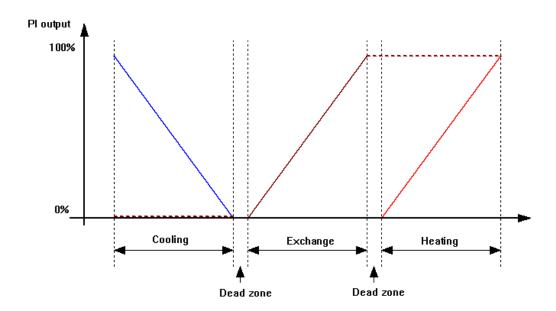
Neutral zone (dead zone) may be used to maintain a desired temperature with a *Tset dead zone* parameter. For example, if the set desired temperature is 22°C and *Tset dead zone* is set to 2°C, then the desired temperature for heating is 21°C, and for cooling - 22°C.
