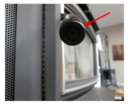
Unscrew 7/64" Allen Key screw counterclockwise. Once the screw is completely loose, remove and drop the handle down off the door handle shaft and replace with new handle.
