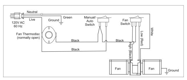
Blower/Fan Wiring Diagram
