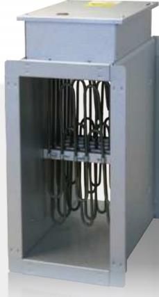
Rectangular electric heaters EKS are designed to heat clean air in ventilation systems. Casing is made from aluzinc coated steel which is high temperature proof. Heating elements tube is made from stainless steel AISI 304. In heaters are installed 2 protection thermostats, screw terminals for easy connection. All EKS duct heaters has two-stage overheat protection.
